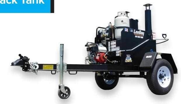
The 150 Tack Distributor ideally serves the paving contractor dedicated to smaller projects. With a conservative 150 gallon capacity tank, this solution still boast of many features and functions of the larger units. Inclusive of a powerful Honda engine, the userfriendly design can either be trailer or skid mounted. Multiple additional options including in-cab controls or overnight heating can further enhance the end user's experience.
